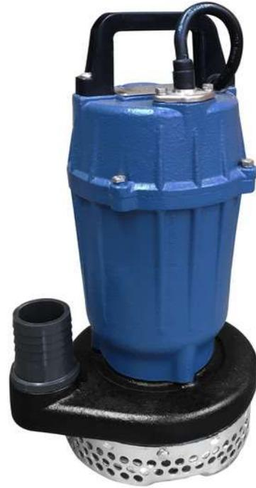
The SS6-9 is a rugged, cast iron cased, electric submersible pump, powered by a single phase, 0.4 Kw, 240Vdc, 50Hz induction motor drawing 3.9 Amps. Optimum performance being 6m3 / Hr at 9Mts head.
